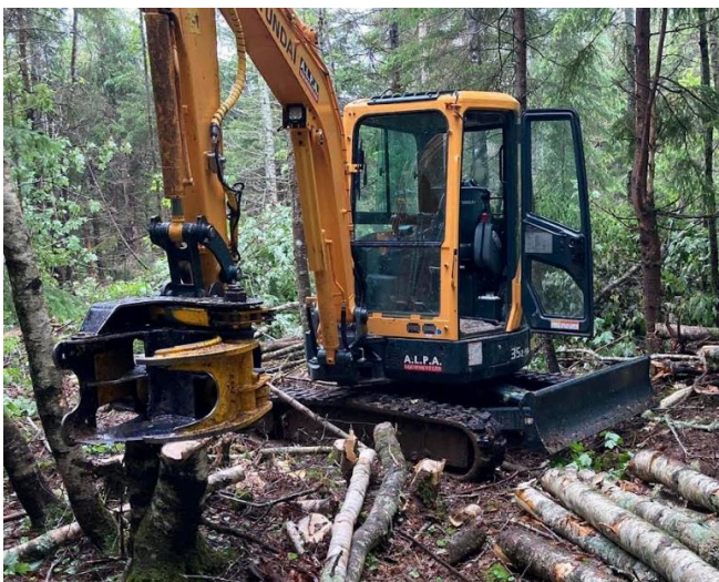
Fig. 1. A small, tracked excavator with shearing-head that is potentially suitable for restoration thinning work.
