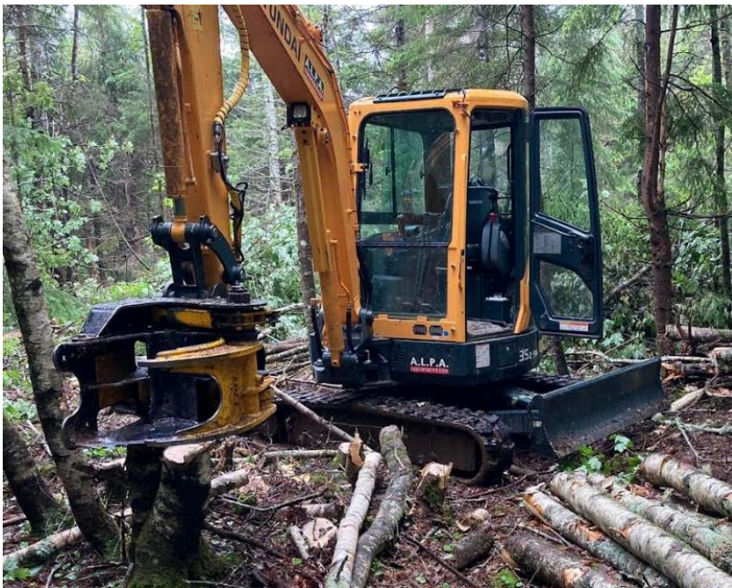
Fig. 4. A small, tracked excavator with shearing head suitable for tall PCT work.
